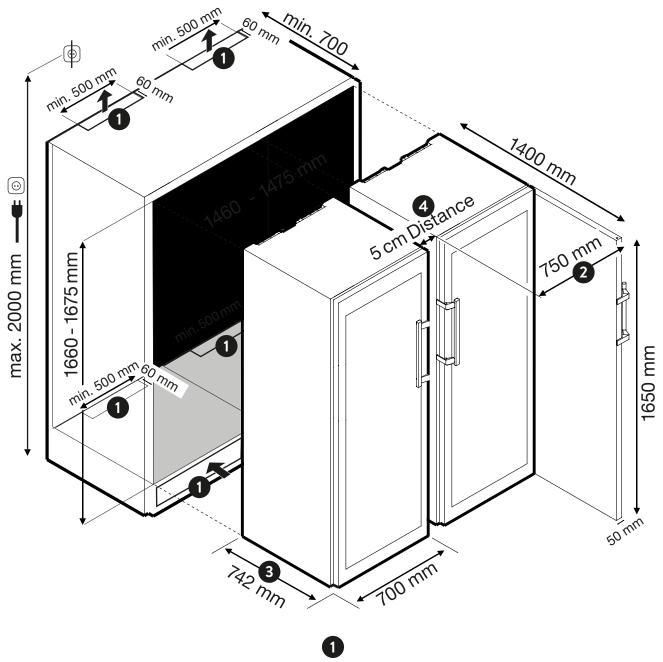
It is absolutely essential to have good air circulation around the unit. Minimum **Height: 300 cm² per device**.
